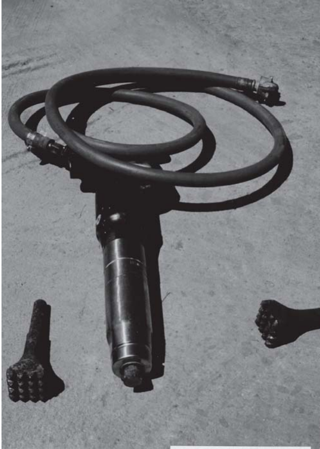
Figure 8-5. Tool used for bush hammering concrete surface
