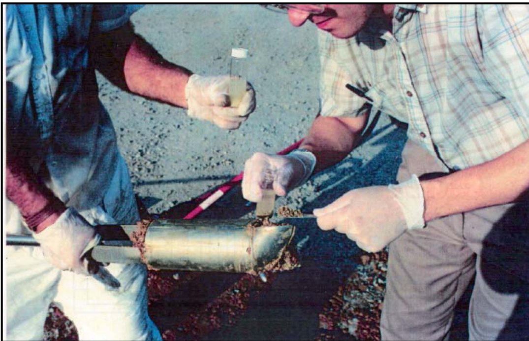
VOC samples should be containerized/preserved immediately on retrieval, or collected directly into the container.
