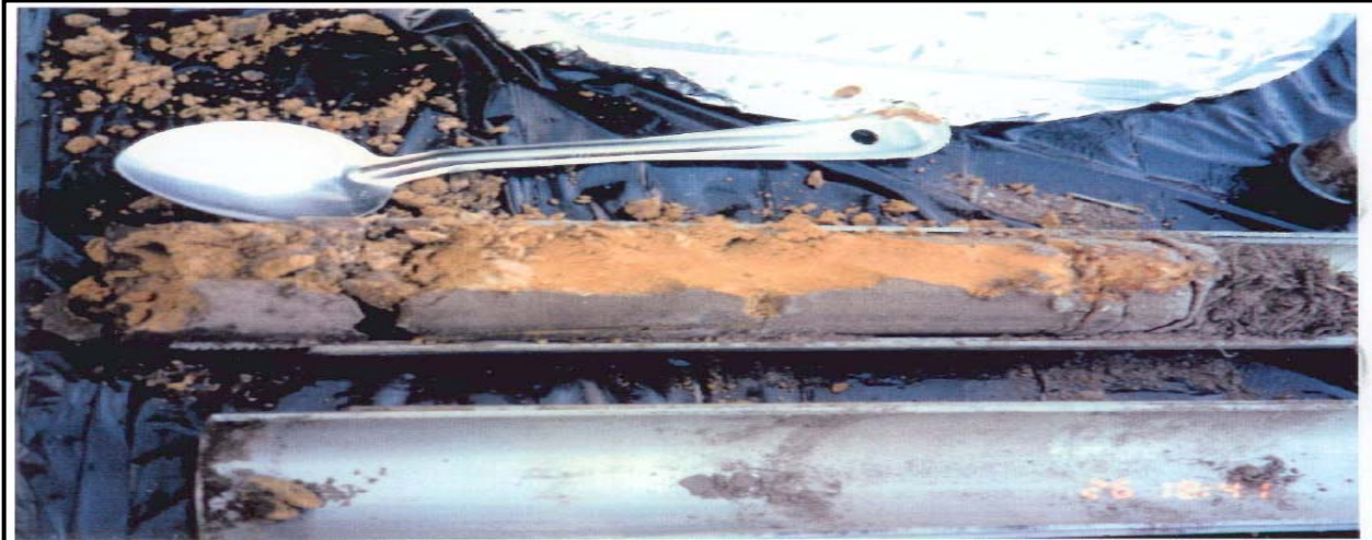
Subsurface samples should be collected in a manner that prevents cross-contamination from surface material. Smearing from 2 inches of gray surface material (right) is seen down the length of a 2-ft split spoon sample.
