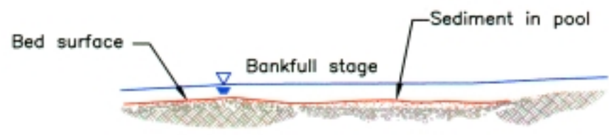
SECTION B - B' - Degraded Condition
