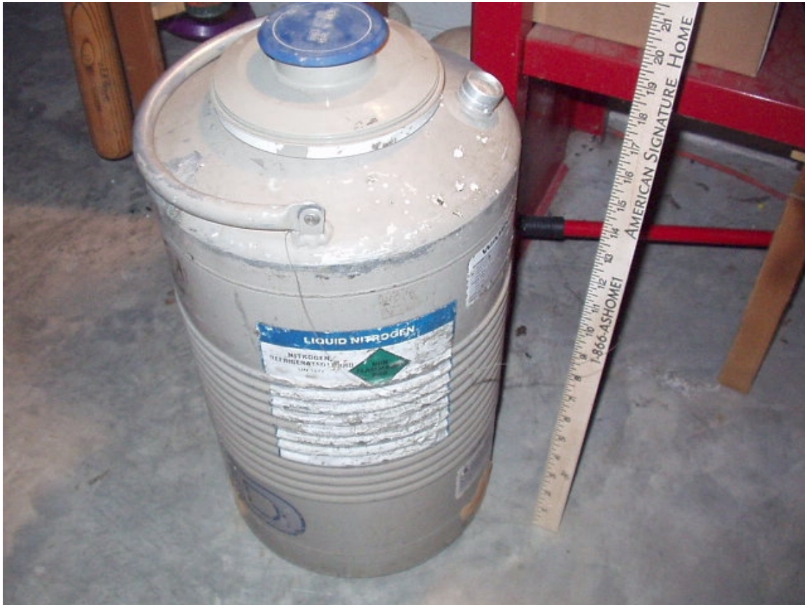
Figure 1. A 10 liter LN 2 container from Airgas (931-645-8276) in Clarksville, TN. As the LN 2 warms, it changes back into the gas state. The loose fitting top prevents explosion. The LN 2 lasts a surprisingly long time (several days) in this type/size container.
