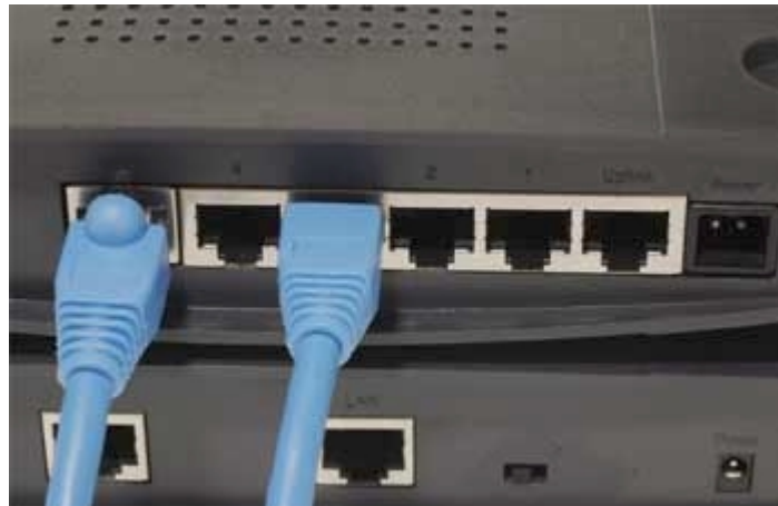
Figure 21. Back of the Linksys Etherfast Router Courtesy of Linksys [2]
