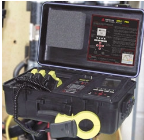
A typical 3-phase power-meter and logger
