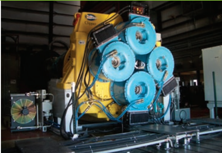
Clipper's new 2.5-MW turbine features an innovative distributed drivetrain.
