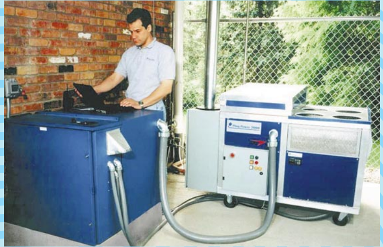
The world's first prototype polymer electrolyte membrane fuel cell (on the right) used to provide all residential power needs for a home in Latham, New York. This 7kW unit is attached to a power conditioner/storage unit that stores excess electricity. (Courtesy: Plug Power)
