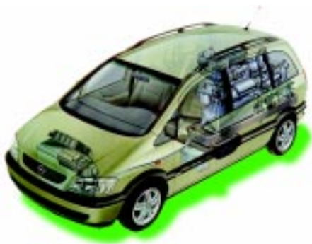
The Opel Zafira, by General Motors, reforms methanol to operate a polymer electrolyte membrane fuel cell. This vehicle has nearly zero emissions of sulfur dioxide and nitrogen oxides and the carbon dioxide output is expected to be 50% less than a comparable internal combustion engine vehicle. (Courtesy: General Motors)
