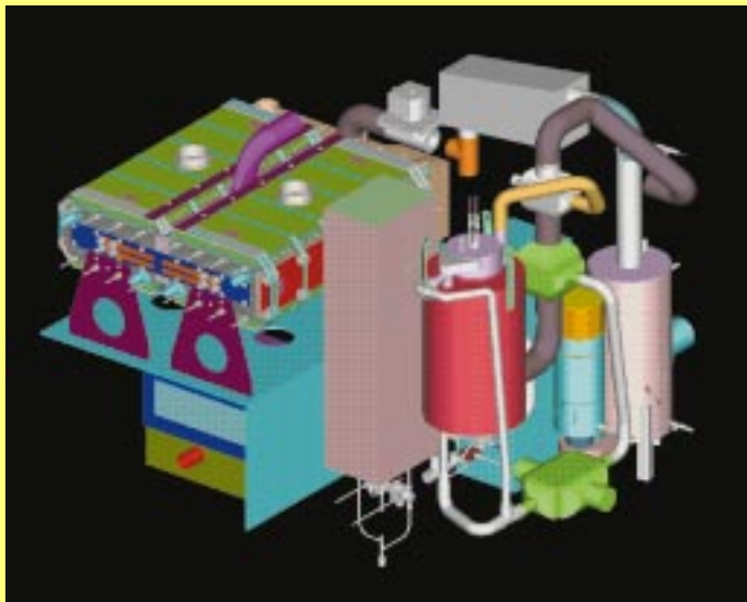
Computer model of 50kW fuel cell stack with reformer. (Courtesy: International Fuel Cells)
