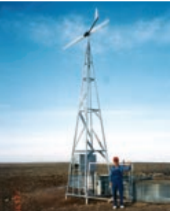
Location—A ranch near Wheeler, Texas Capacity—1 kilowatt Turbine manufacturer—Southwest WindPower Photo Credit—Elliott Bayly/PIX07169
