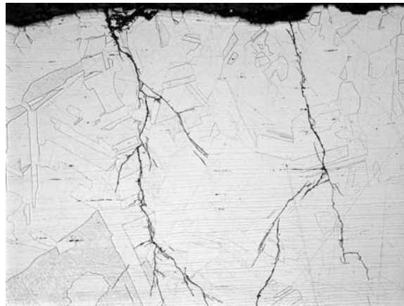
Micrograph showing transgranular SCC in Stainless Steel
