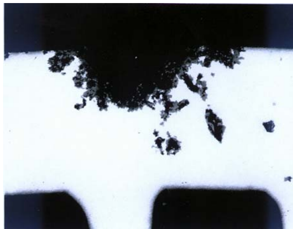
Micrograph showing pit "network"
