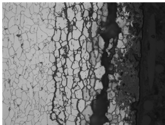
Micrograph showing intergranular attack
