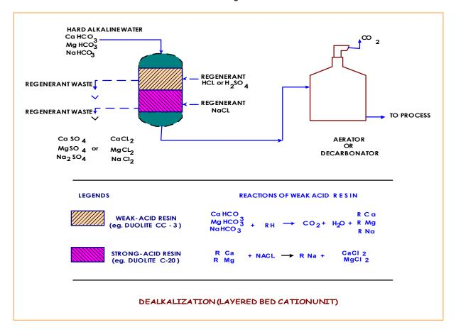
Note that the dealkalizer would seldom be used without a base-exchange softener, as the solution produced is acidic and would cause corrosion, and any permanent hardness would pass straight into the boiler.
