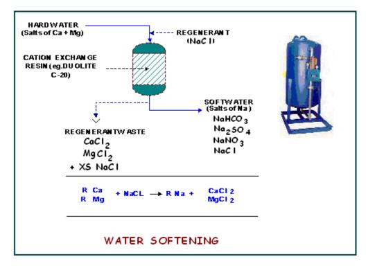
A softener will continue to produce *soft* water as long as there are sodium ions remaining on the resin to "exchange" with the calcium & magnesium ions in the *hard* water. When the supply of sodium ions has been depleted, the resin must be *regenerated* with a new supply of sodium ions.
