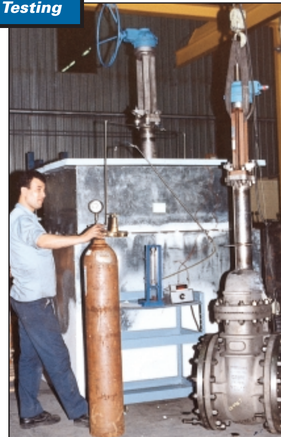
Cryogenic test bench
