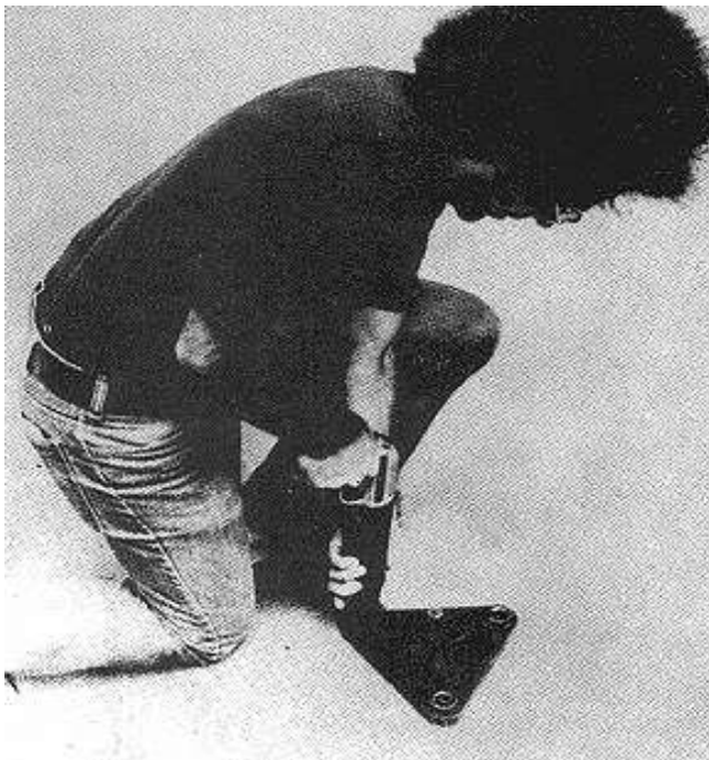
Figure 2-37. Windsor probe in use
