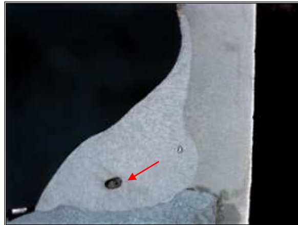
Figure 4. Fillet weld section showing porosity
