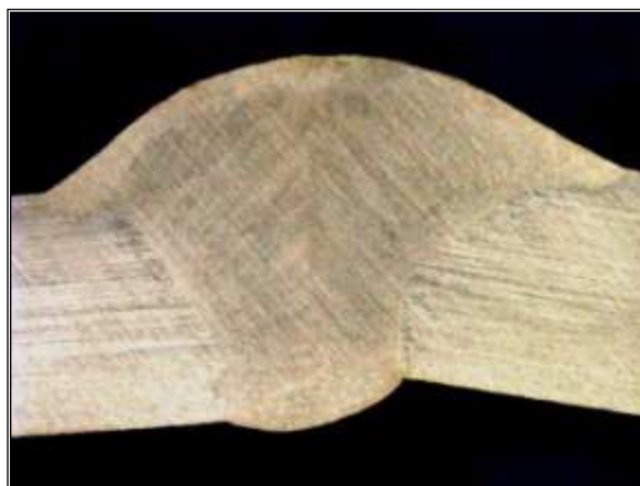
Figure 17. Macrograph showing poor fit-up (butt weld)
