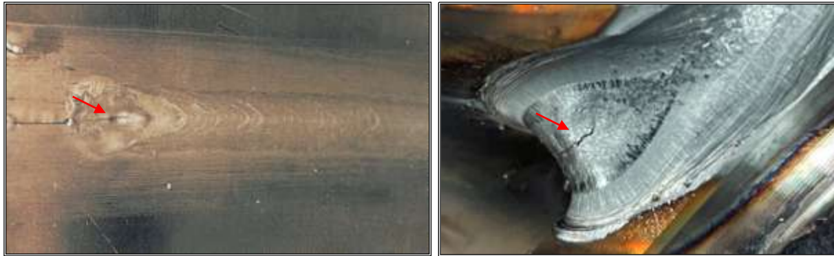
Figure 20. Photographs illustrating crater cracking resulting from abrupt weld termination in an aluminum weld on left, steel on right (MIG process). These cracks occur due to shrinkage stresses that develop as a result of rapid cooling of the crater compared to the remainder of the weld bead.
