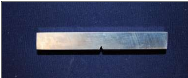
Figure 32. Photograph showing a notched charpy impact specimen ready for testing
