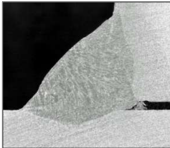
Figure 8. Acceptable fillet weld
