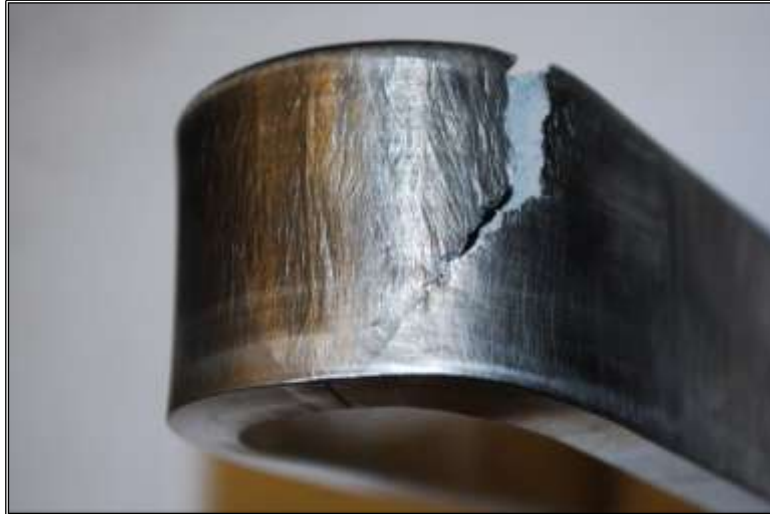
Figure 30. Photograph of a side-bend sample, which failed as a result of lack of fusion
