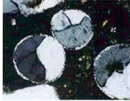
Air Voids Filled with Gypsum
