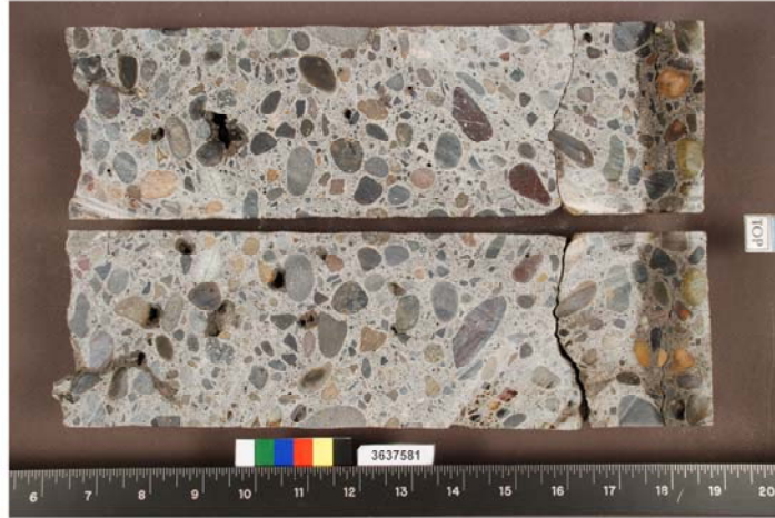
Example of Consolidation of Concrete Sample
