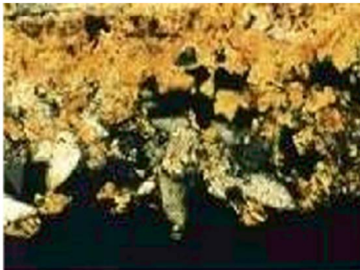
Gypsum Crystals at an Exterior Surface Placed against Soil
