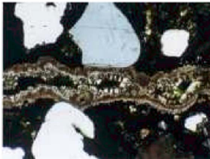
Magnesium Hydroxide Formation in a Crack
