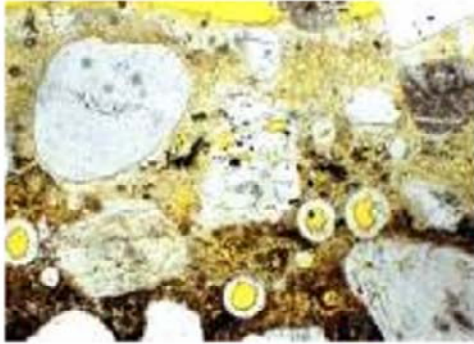
Cement Paste Turned into Gypsum
