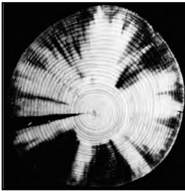
Figure 14–2. Typical radial penetration of log by stain. The pattern is a result of more rapid penetration by the fungus radially (through the ray) than tangentially.
