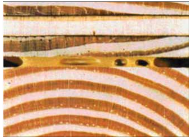
Figure 10-12. Gap-filling construction adhesive in field-assembled plywood floor system.
