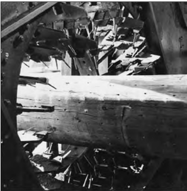
Figure 15-4. Deep incising permits better penetration of preservative.
