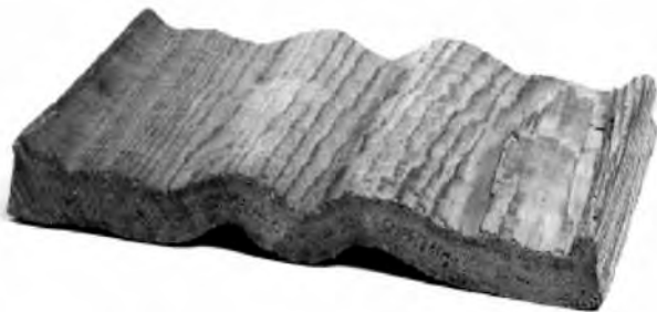
Figure 13-10. Severe collapse in western redcedar.
