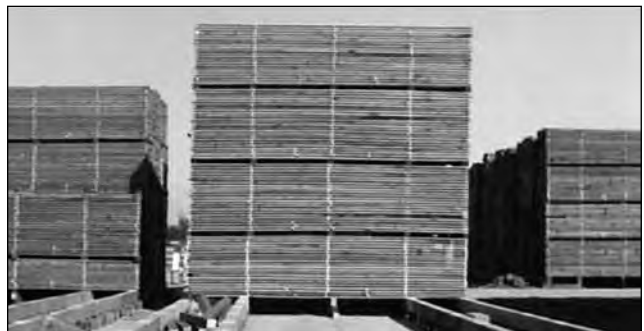
Figure 14–7. A sanitary, well-drained air-drying yard.
