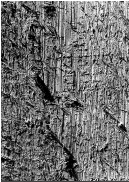
Figure 5-7. Projecting tension wood fibers on sawn surface of mahogany board.
