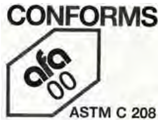
Figure 11-12. Typical grade stamp for cellulose fiberboard. (Courtesy American Fiberboard Association, Palatine, Illinois. Used by permission.)
