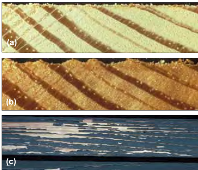
Figure 16-22. (a) Cross-section view of flat-grain southern yellow pine showing dense LW bands crushed into less dense EW directly beneath them; (b) raised grain caused by rebound of LW bands following wetting; (c) a thin coat of film-forming finish applied over a stressed flat-grain surface will crack as the wood rebounds.
