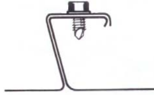
Sidelap Screw Connector Source: Bondek
