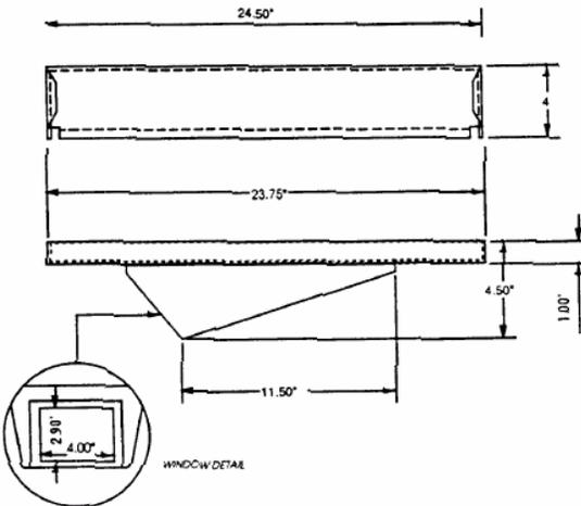
The PRC-201C housing is designed for use in suspended or sheet rock ceiling applications. Units are sized for use with a solid state 1/8" or 1/4" camera and lens combination. Housings are manufactured from 94HB flame rated plastic, with viewing windows manufactured from high impact optically clear acrylic. PRC-201C is fully adjustable for 360° positioning. Units includes 26-gauge galvanized steel metal cover.
