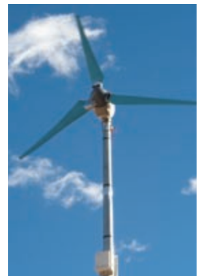
Southwest Windpower's 1.8-kW prototype turbine.
