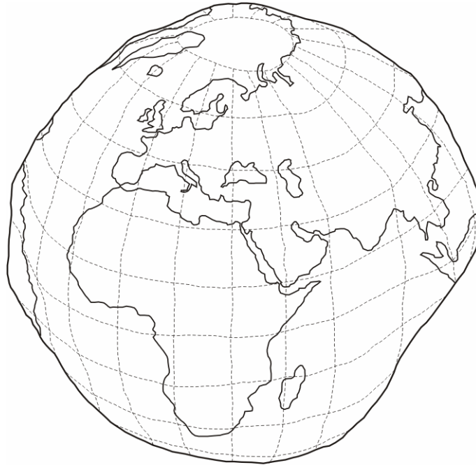
Figure 3.7 Exaggerated representation of the geoid.
