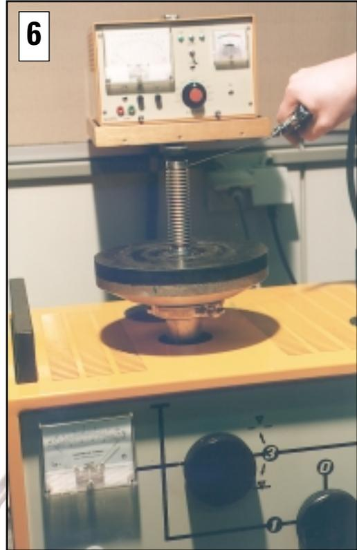
6 Helium leak testing. Bellows are rejected if leakage exceeds  $10^{-8}$  cm<sup>3</sup> per second.
