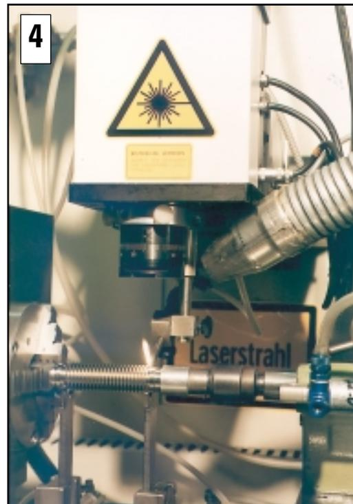
Laser welding of bellows to end rings.
