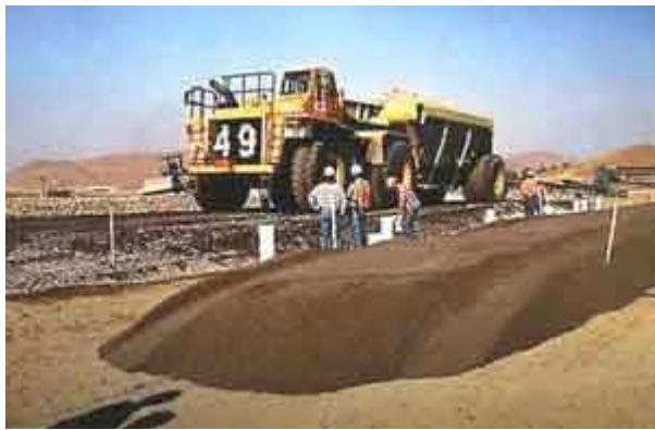
Figure 10: This example shows large scale field testing of a fill sample to verify grading, moisture content and compressibility before using the material in the construction of a dam.
