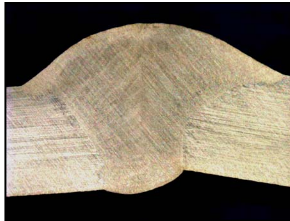
Macrograph showing poor fit-up (butt weld)
