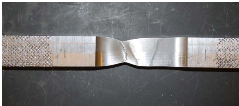
Photograph of an acceptable transverse weld tensile specimen that failed in a ductile manner, in the base metal
