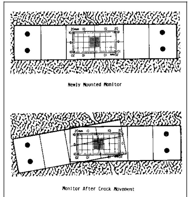
Figure 2-33. Crack monitor
