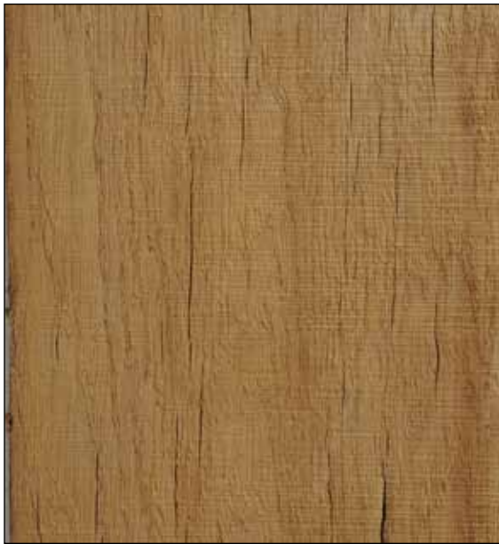
Figure 13–8. Surface checking on white oak 5/4 lumber.
