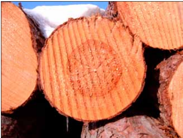
Figure 13–9. End checking in red pine logs.
