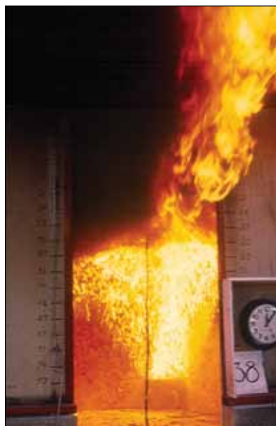
Figure 18-1. Flashover in standard room test.
