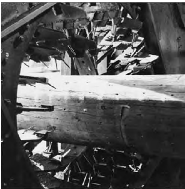
Figure 15-4. Deep incising permits better penetration of preservative.
