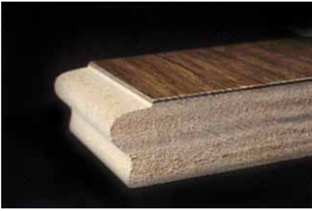
Figure 11–13. Medium-density fiberboard with veneer overlay. Edges can be shaped and finished as required by end product.
